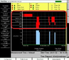
CRC, or the Cyclic Redundancy Check numbers, are included in the Extended Super-Frame (ESF) format. If the received CRC and the CRC calculated from the received data do not agree, the received data must be in error.
